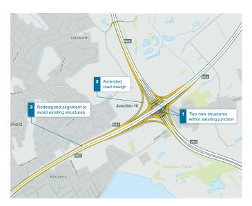
The changes we made to refine Option C into the Inner Links option are as follows:
